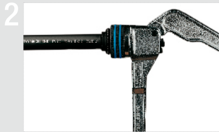
Expand the pipe
